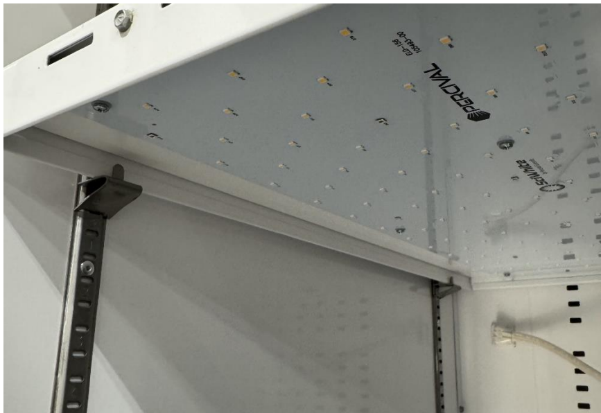
(Tabs on pilaster clips must sit inside lamp bank flanges)
