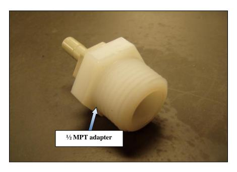
(Optional) ½ MPT adapter. Insert into compression fitting and connect water supply with ½ FPT fitting
