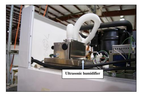
Periodically check the discharge from the humidifier (while the Intellus controller is calling for humidity) to verify that the humidified air produced is composed of very fine water droplets. The proper humidity rich air discharged from the ultrasonic humidifier is composed of very small water droplets and looks like fog or smoke. The production of large water droplets or no water droplets at all could signal a malfunction in the humidifier.
